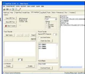
⇒ The Garmin protocol is not selected on the GPS. EasyPlan reports "Port Open" and "Msg Sent 0" but gets no response. This indicates the GPS is not connected to the port, or is set on the wrong protocol. See the GPS Operating Instructions.
